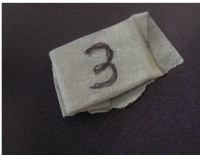
Figure 6.7: The TLD covered with plastic cover, wrapped by masking tape with its unique number.
