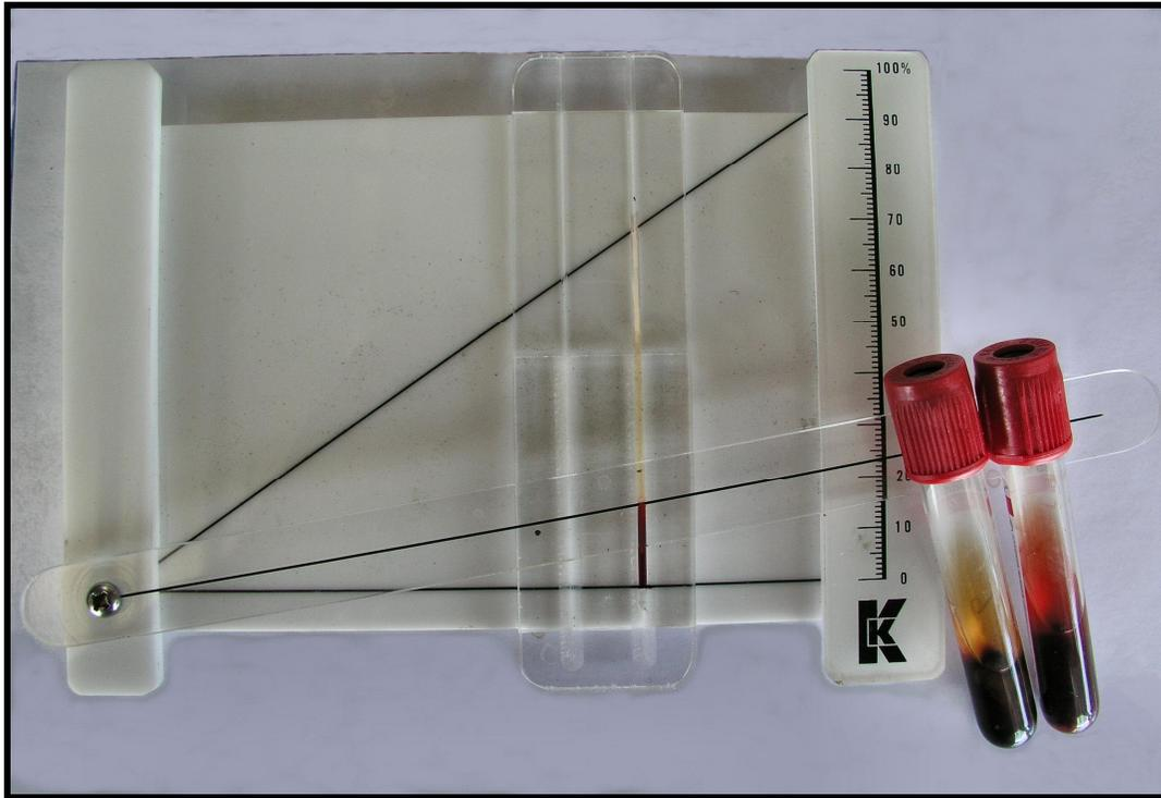
**Figure 2.8:** The hematocrit reader with capillary tube and blood samples for protein determinations.
