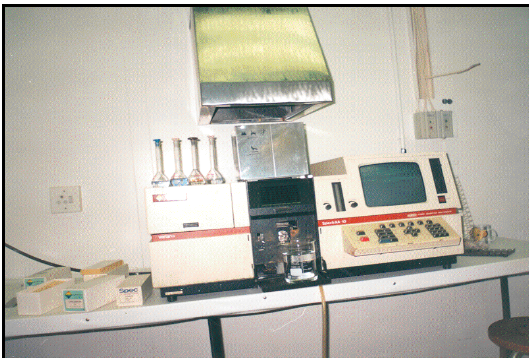
Figure 3.2 Atomic Absorption Spectrophotometer (AAS) Spectr AA. 10 plus.
