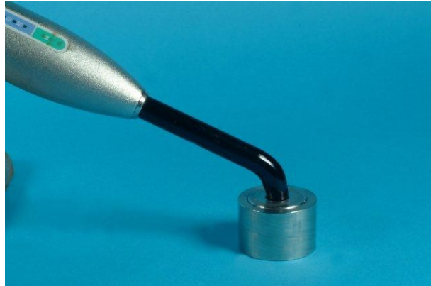
Fig. 15: Elipar Freelight 2 curing light in light guide alignment ring
