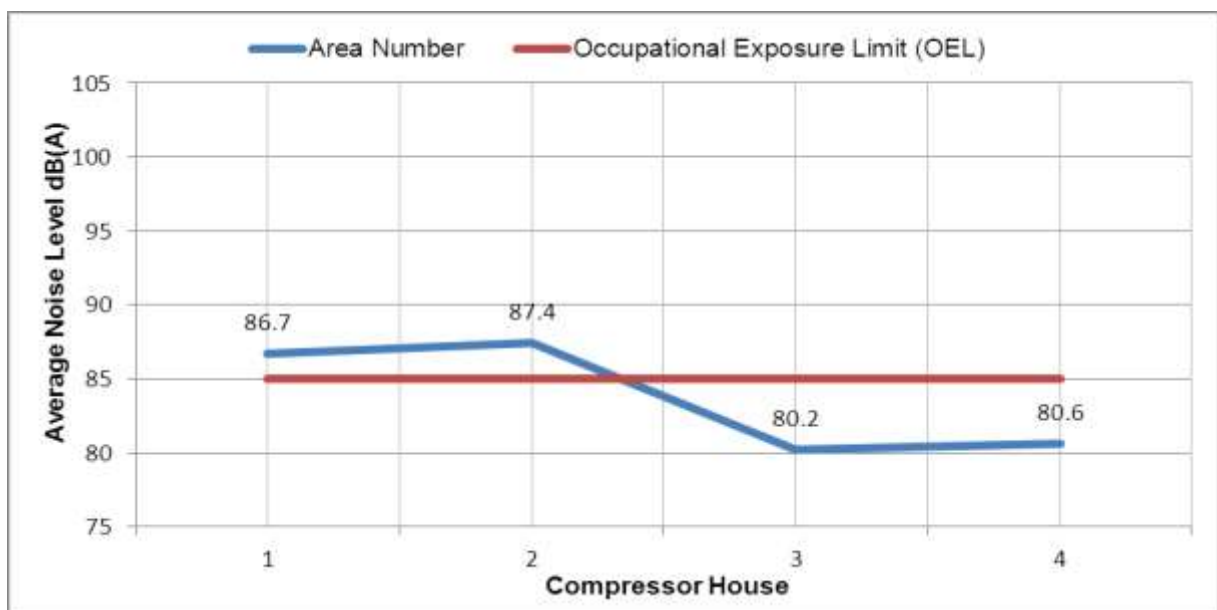
Figure 2: Average noise level at the four areas at the Compressor House.
