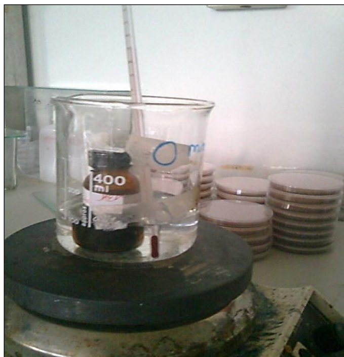
Figure 3.7: The process of water dis-infection from bacteria at controlled temperature.
