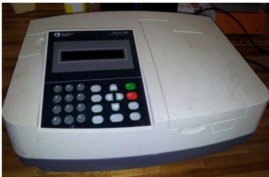
Figure 3.4: UV/Vis spectrophotometer used to analyse 4-hydroxynitrobenzene samples.
