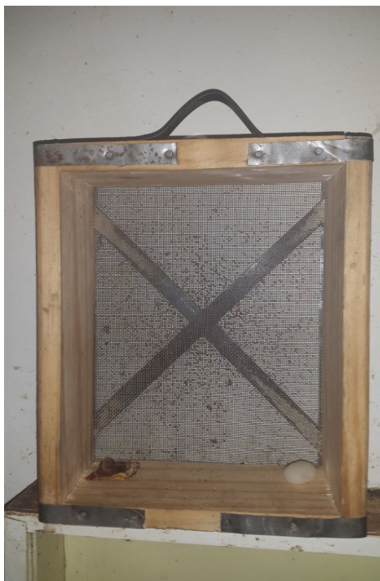
Figure 3: A traditional beer strainer is suitable for measuring the particle size of the sawdust (Source by author)
