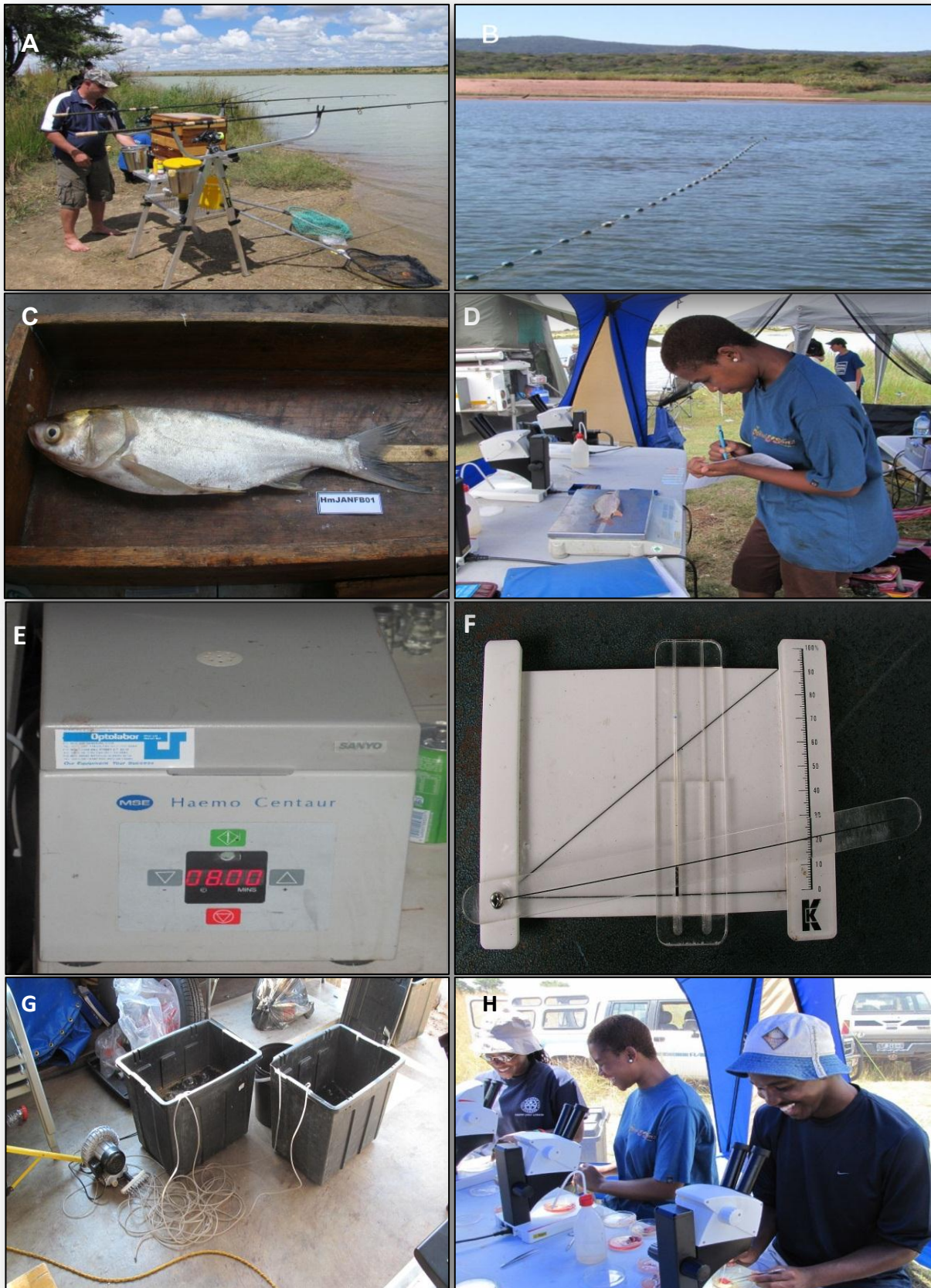
Figure 2.6: Health assessment. A- conventional angling gear and scoop nets; B- gill nets; C- calibrated measuring board; D- Salter Model 235E electronic balance; E- micro-haematocrit centrifuge (model: KHT-400); F- micro-haematocrit reader; G- aerated holding tanks; H- examination of fish organs in a field laboratory.
