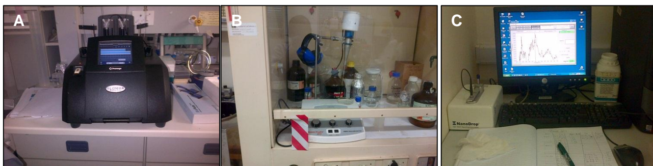
Figure 2.8: Oxidative stress biomarker analysis. A- Glomax ® Multi Microplate Multimode Reader; B- Omni-Ruptor 400; C- NanoDrop.
