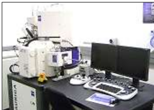
Figure 20: The SEM instrumentation – Auriga Cobra FIB FESEM – made available by the CSIR.
