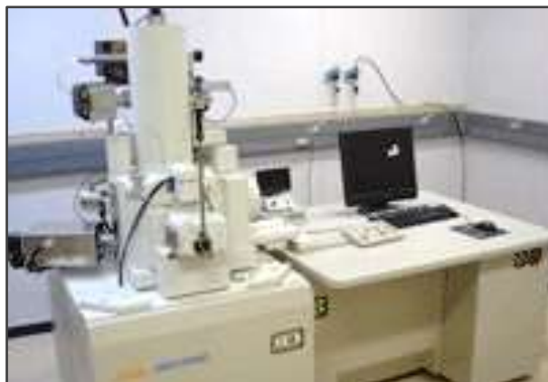
Figure 22: The EDS instrumentation – JEOL JSM-7500F FESEM / ThermoScientific UltraDry EDS – made available by the CSIR.
