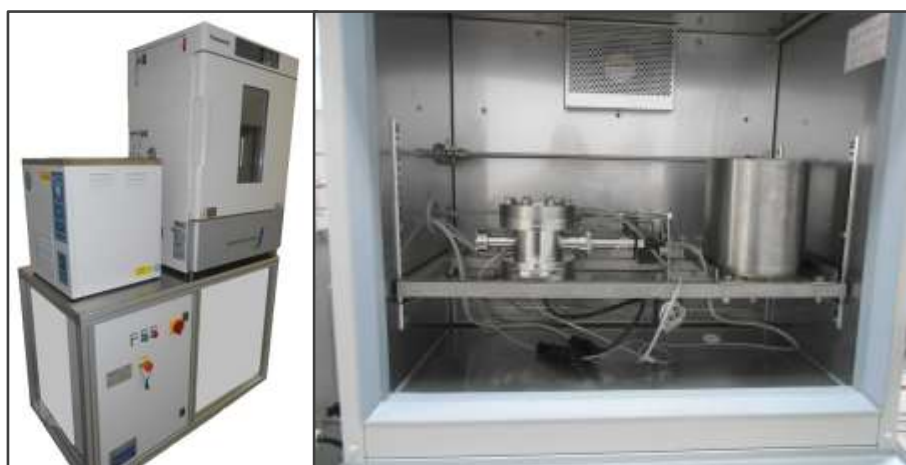
Figure 29: Gas sensor testing system by Kenosistec [291].
