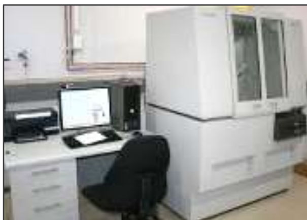
Figure 17: The XRD instrumentation – PANalytical X'Pert PRO diffractometer – made available by the CSIR.
