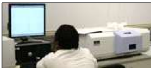
Figure 26: The UV-vis instrumentation – Perkin-Elmer LS 55 Fluorescence Spectrometer – made available by the CSIR.
