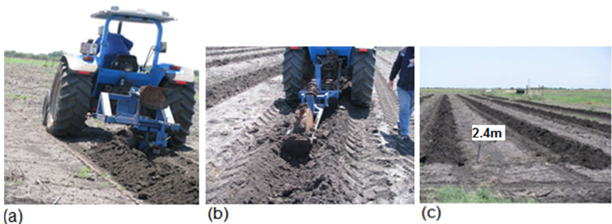
Figure 3.2 The IRWH implements; furrow plough (a), basin maker (b) and created basins (c).
