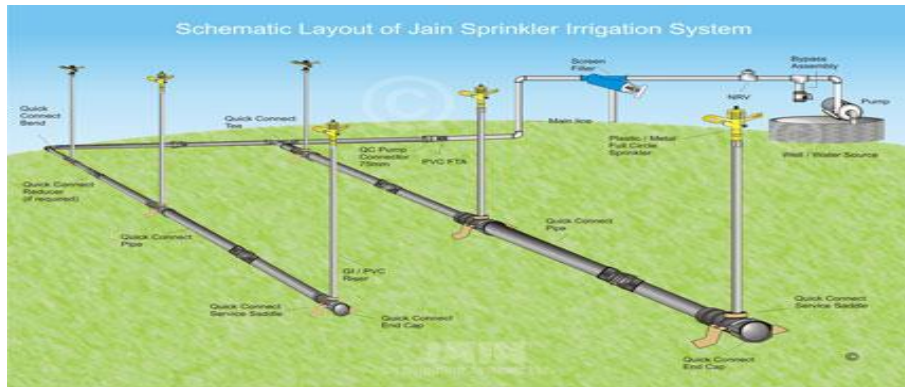
Figure 2.1: A picture of schematic layout of irrigation pipes in a field ( www.shutterstock.com .)
