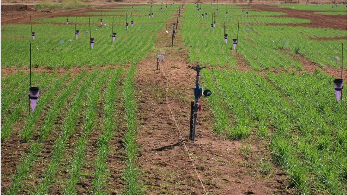
Fig. 9.1: Photo taken from the field showing the rain gauges, sprinklers and Diviner 2000 access tubes
