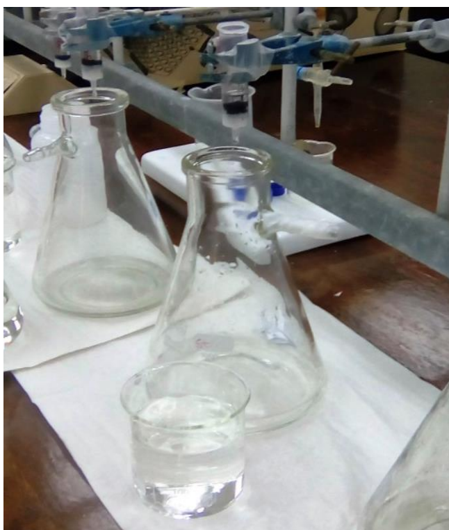
Figure 3.10: Set up for off-line application of SPE
