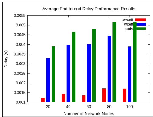
Figure 5-20: The average latency versus the number of cognitive radio nodes
