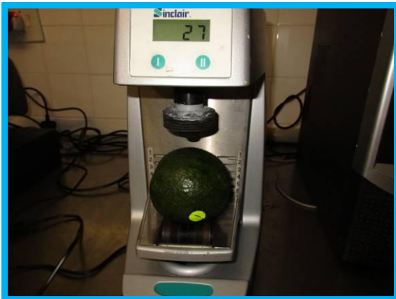
Figure 3.2 Sinclair IQ™ automated desktop firmness machine used to measure fruit firmness of 'Reed' avocado fruit.
