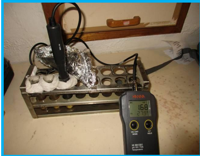
Figure 3.5 Electrical conductivity EC meter used to measure electrolyte leakage
