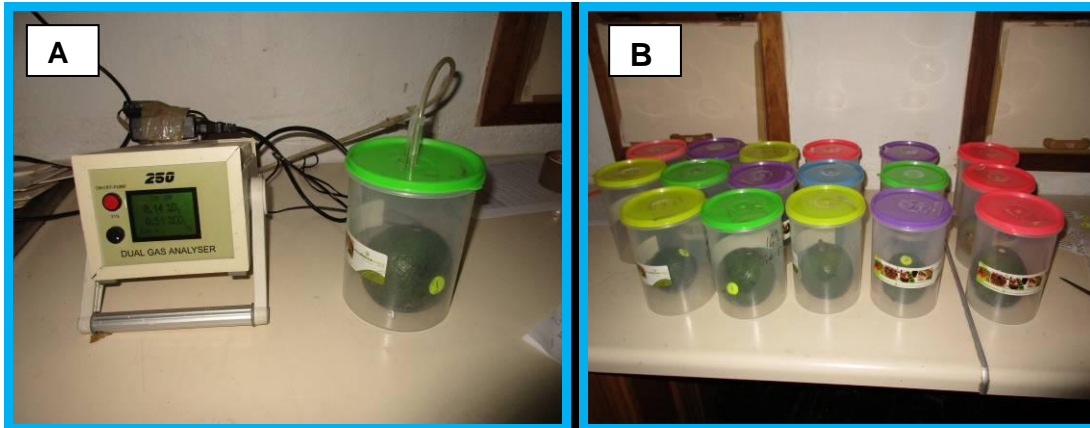
Figure 3.3 Infrared gas analyzer measuring CO 2 evaluation (A) and individual 'Reed' avocado fruit Incubated in 1 L plastic jar (B)
