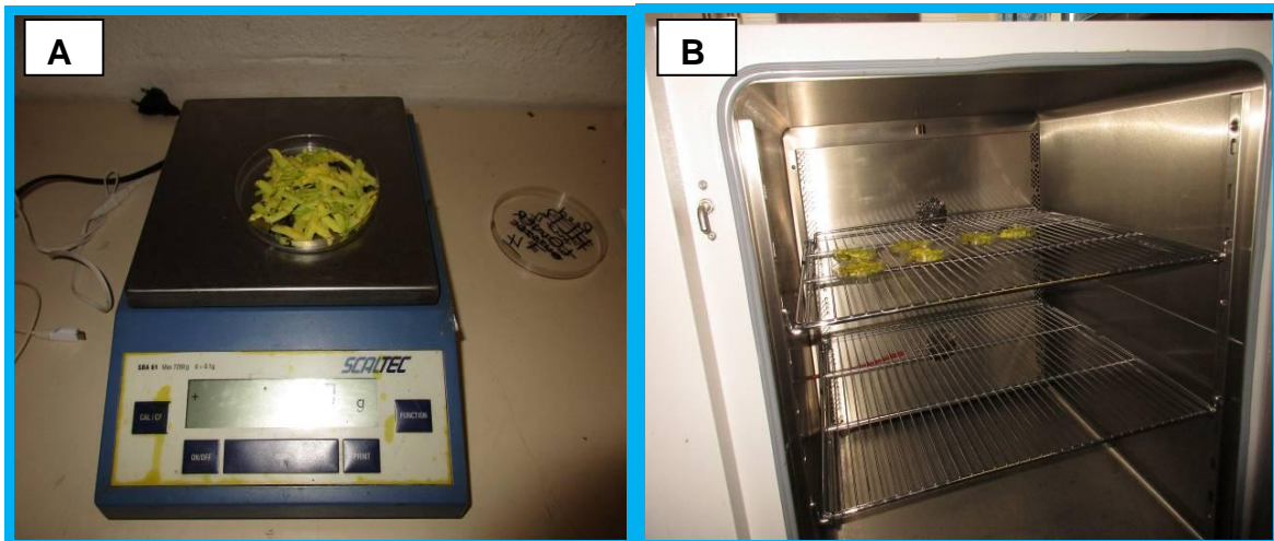
Figure 3.1 Weighing scale measuring flesh sample mass (A) and oven drying fruit flash of 'Reed' avocado fruit (B)
