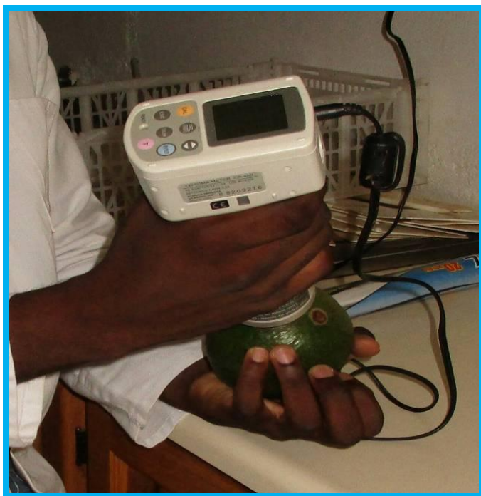
Figure 3.4 Chromameter used to measure colour parameters Lightness ( L^* ), a^* and b^* values)
