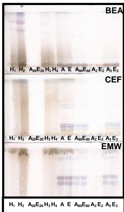
Figure 3.10: Chromatograms developed in BEA, CEF and EMW, then sprayed with vanillin-sulphuric acid reagent. n-Hexane wash for acetone ( H_1 ), n-hexane wash for ethanol ( H_2 ), 20% acetone wash ( A_{20} ), 20% ethanol wash ( E_{20} ), n-hexane wash for 20% ethanol ( H_3 ), n-hexane wash for 20% acetone ( H_4 ), acetone extract pre-treated with n-hexane ( A ), ethanol extract pre-treated with n-hexane ( E ), 80% acetone extract pre-treated with 20% acetone ( A_{80} ), 80% ethanol extract pre-treated with 20% ethanol ( E_{80} ), 20% acetone wash for n-hexane pre-treated material ( A_2 ), 20% ethanol wash for n-hexane pre-treated material ( E_2 ), acetone extract for materials pre-treated with 20% acetone and n-hexane ( A_3 ), ethanol extract for materials pre-treated with 20% ethanol and n-hexane ( E_3 ).
