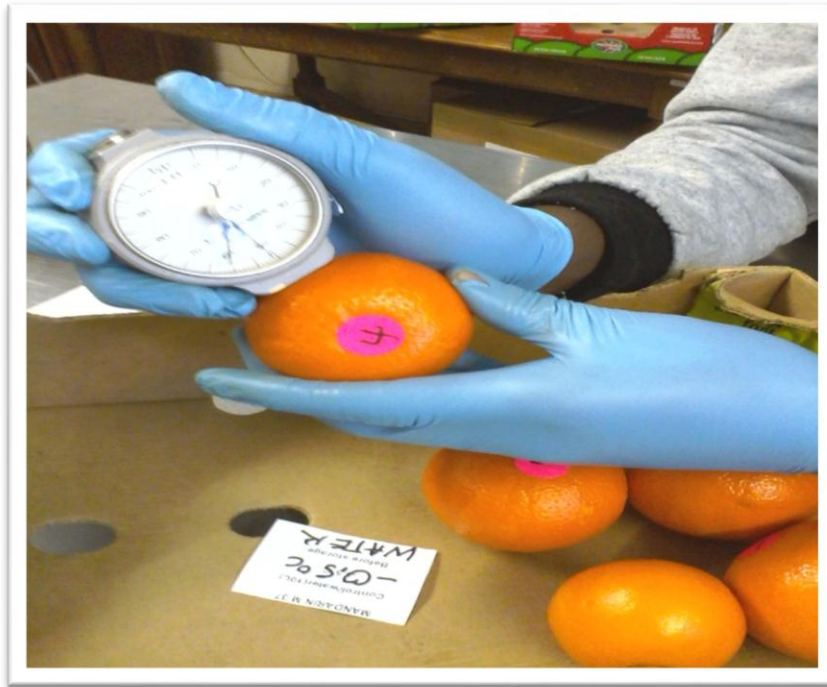
Figure 3.2 Densimeter used to measure fruit firmness.
