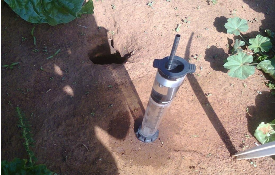
Figure 2: Infiltration rate determination.
