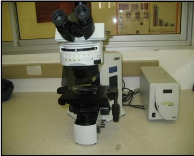
Figure 4.4. Fluorescent microscope used for spermatozoa morphology evaluation
