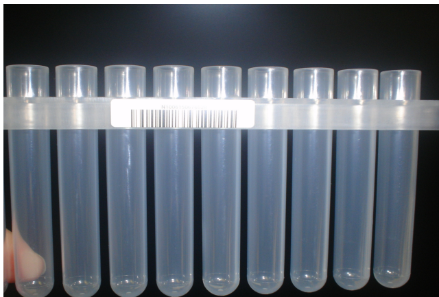
Figure 2.2 Bar-coded Ten-Tube Unit (TTU).
