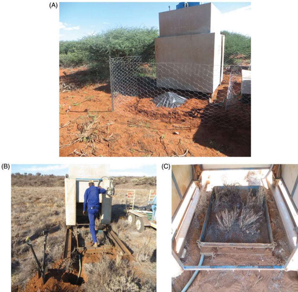
Figure 3. Hofrey rainfall simulator (A) being mounted on the experimental plot (B) fitted with a 1\text{m} \times 1\text{m} metal frame and surface runoff collecting pipe (C).
