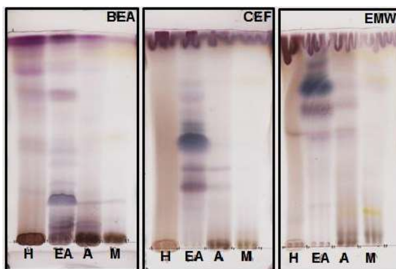
Figure 3.14: Chromatograms of phytochemical constituents from S. pinnata extracts separated in BEA (left), CEF (middle) and EMW (right) solvent systems and sprayed with vanillin sulphuric acid reagent. Lanes from left to right: n-hexane (H), ethyl acetate (EA), acetone (A) and methanol (M).
