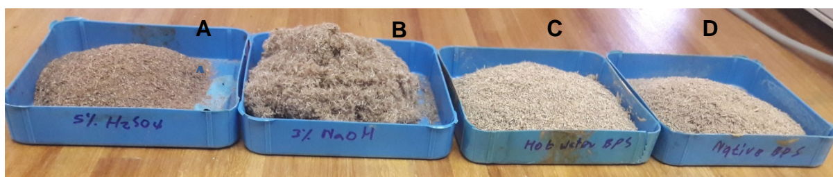
Figure 5.1. Banana pseudostem before and after different pretreatments. A 5% H 2 SO 4 , B 3% NaOH, C Hot water and D Native (Untreated).
