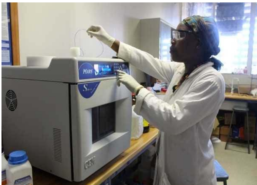
Figure 3.5: Photo depicting the microwave-assisted acid digestion system
