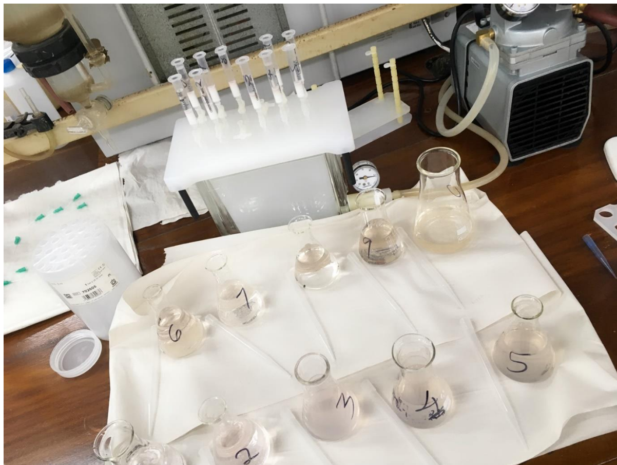
Figure 3.8: SPE set up for sample preparation and application
