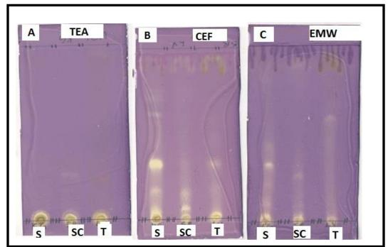
Figure 4: Compounds with antioxidant activity on TLC plates in *Seriphium plumosum, Schkuhria pinnata* and *Toona cilliata* developed with TEA (A), CEF (B) and EMW (C) as mobile phases. The chromatograms were sprayed with 0.2% DPPH.
