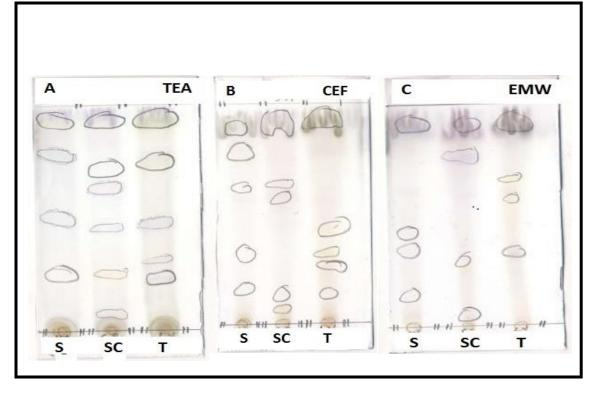
Figure 3: Thin layer chromatograms of acetone leaf extracts obtained from Seriphium plumosum, Schkuhria pinnata and Toona cilliata developed with TEA (A), CEF (B) and EMW (C) as mobile phases. The chromatograms were sprayed with vanillin/H<sub>2</sub>SO<sub>4</sub> and heated in an oven at 110°C for colour development.
