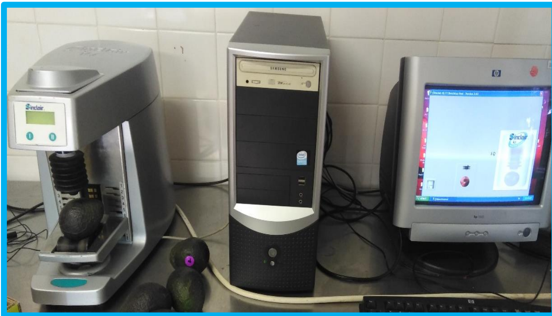
Figure 3.3 Measuring fruit firmness of 'Hass' avocado fruit during ripening
