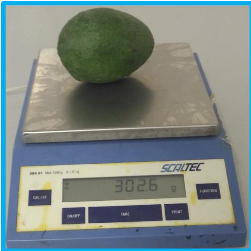
Figure 3.2 Measuring fruit weight of 'Hass' avocado fruit during ripening
