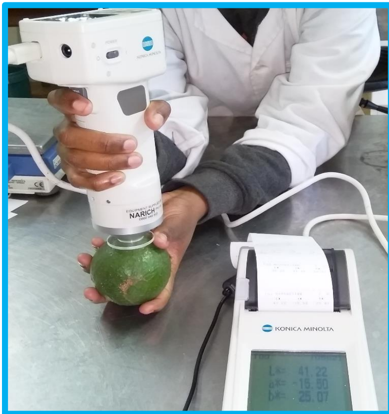
Figure 3.5 Measuring fruit colour parameters of 'Hass' avocado fruit during ripening
