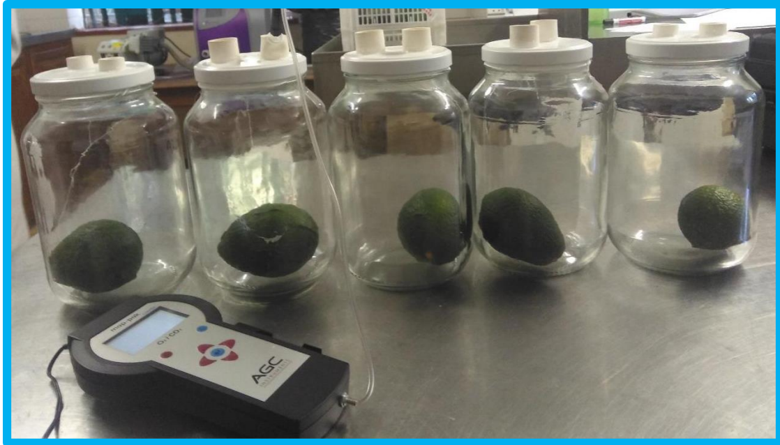
Figure 3.4 Measuring respiration rate ( \text{CO}_2 ) of 'Hass' avocado fruit during ripening
