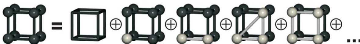
Figure 2-3. A presentation of the decomposition from a cubic lattice into figures that are used in the cluster expansion. The sum has been truncated with regard to the number of vertices as well as possible orientations and shapes of figures with the same number of vertices [106].
