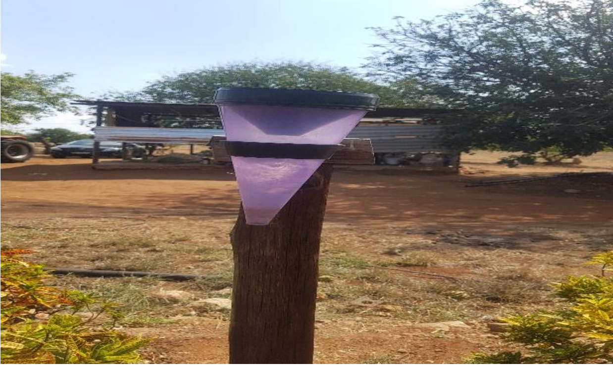
Appendix 5.2. Rain gauge placed at Duvadzi farm and A hi tirheni Mqekwa farm used to measure rainfall volumes.
