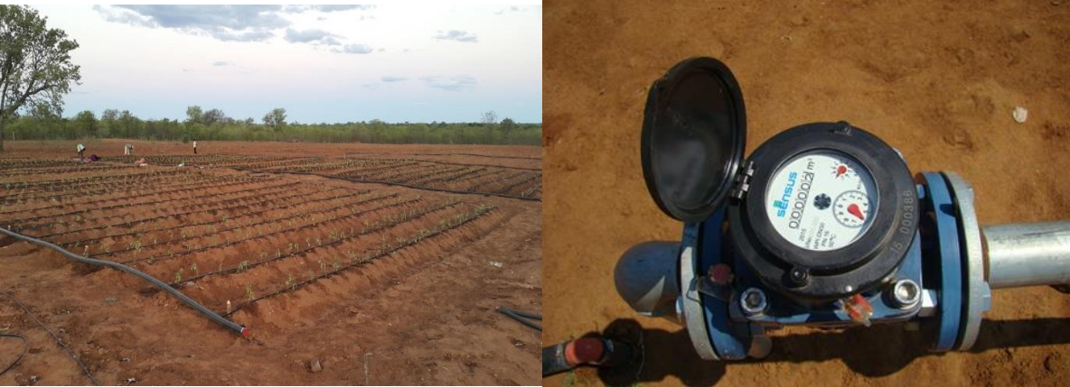
Appendix 5.3 Layout of drip irrigation lines (left) and water volume meter used to measure irrigation volumes (right).
