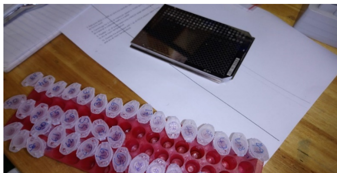
Insert 4.1 A photo showing the MALDI target plate after spotting the supernatant from Eppendorf tubes
