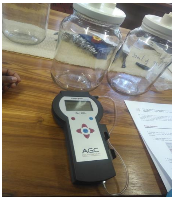
Figure 3.4: Map-Pak gas analyser with glass jar used to measure CO 2 concentration
