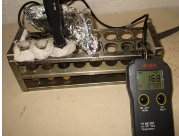
Figure 3.7: Electric conductivity (EC) meter used to measure membrane permeability
