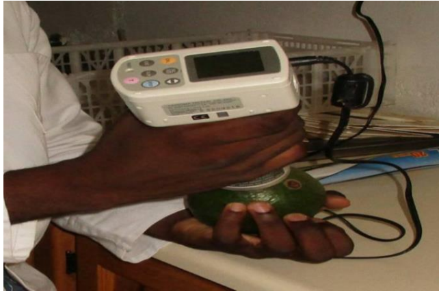
Figure 3.2: Chromameter used to measure objectively hue angle, chroma and peel lightness
