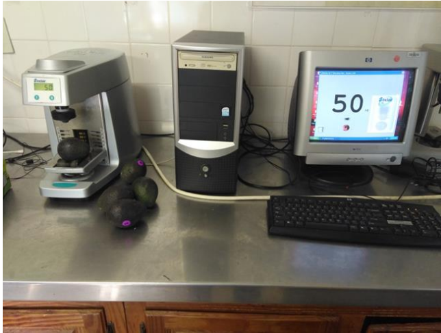
Figure 3.6: Sinclair IQTM desktop firmness machine used to measure fruit softness
