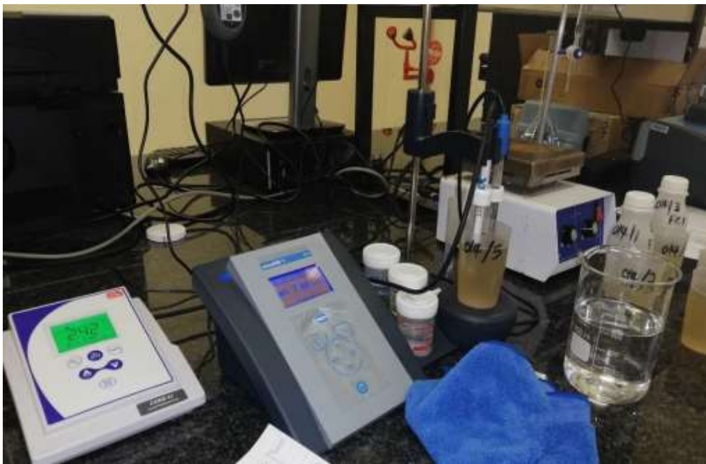
Figure 3.2: A pH and conductivity meter 1120 (Metler Toledo) used to measure pH, conductivity, salinity, and temperature.
