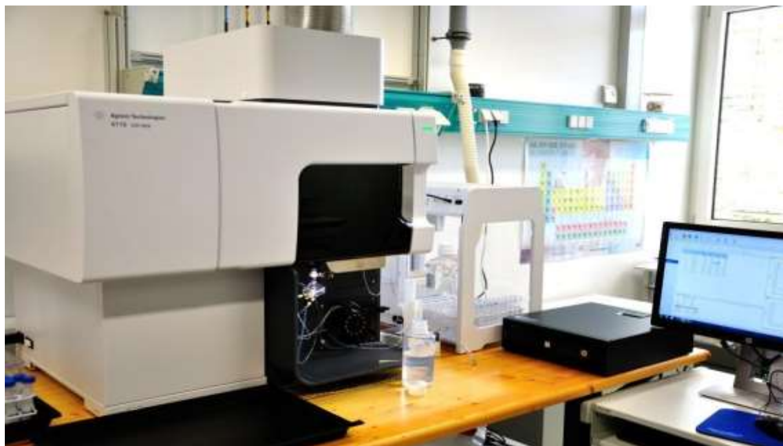
Figure 3.5: A Sequential Type ICP-OES SPS3000 instrument used for elemental analysis.
