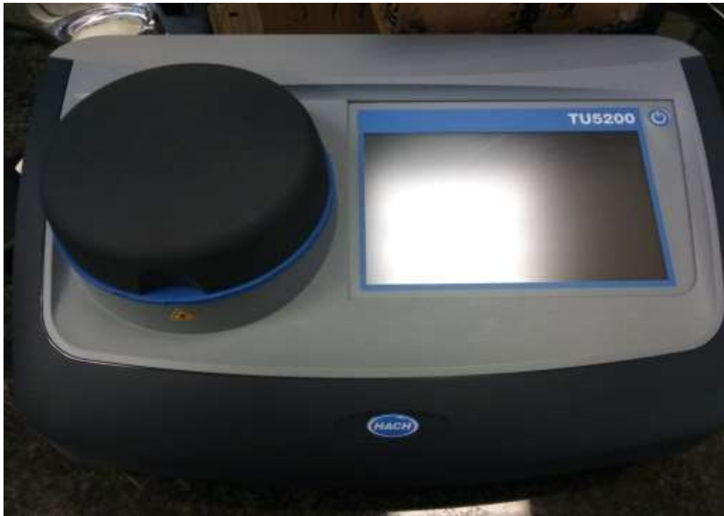
Figure 3.3: A TU5200 turbidimeter used in the analysis of turbidity measured in NTU as the units.
