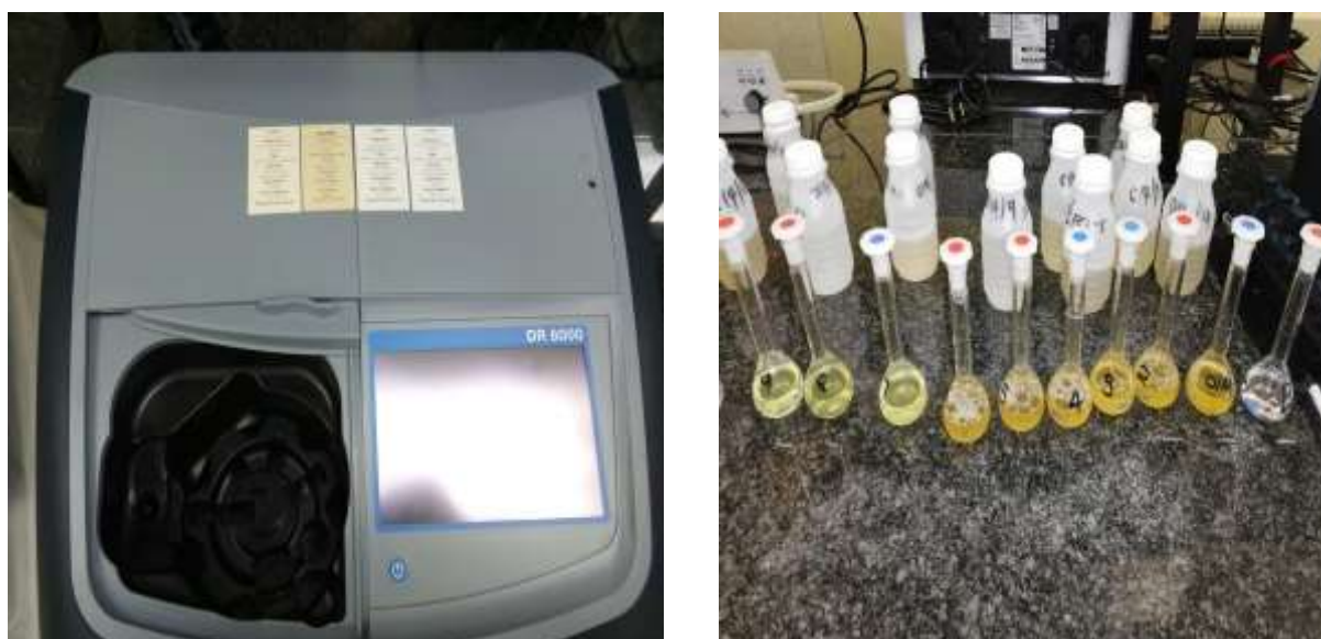
Figure 3.8: A DR 6000 instrument used for ammonia analysis along with the prepared solutions on the right.
