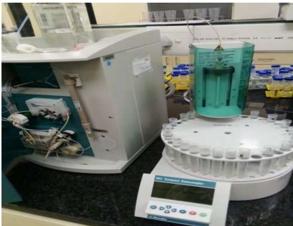
Figure 3.6: A Metrohm 850 Ion Chromatography System used for anions analysis.
