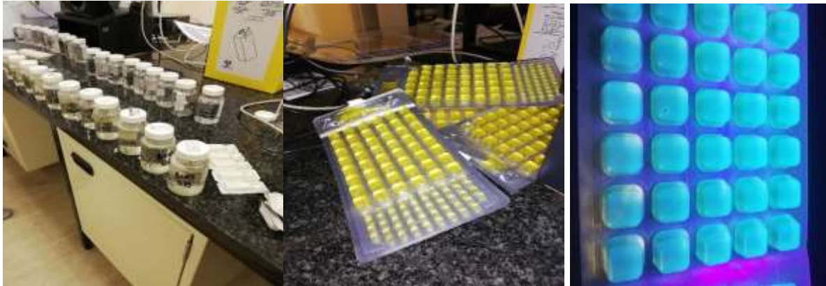
Figure 3.10: A colilert test method used for total coliform and E.coli detection.
