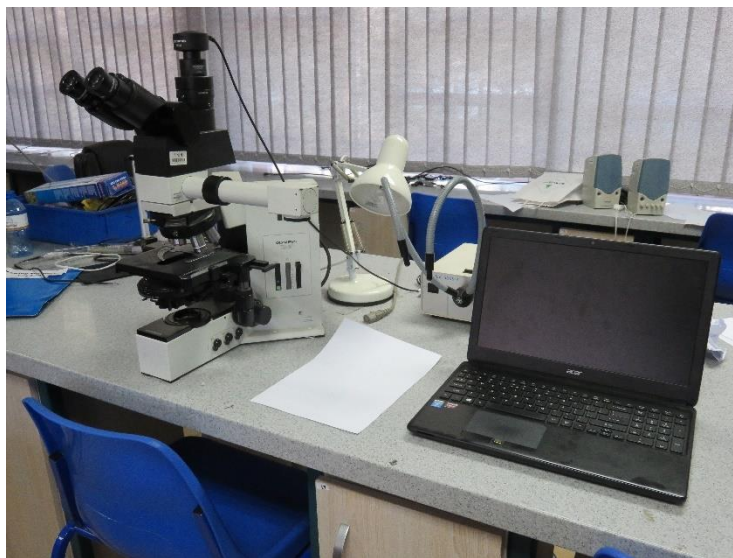
Figure 3.2: Olympus BX50 microscope used in morphological characterisation. (Photograph by Raphahlelo ME)
