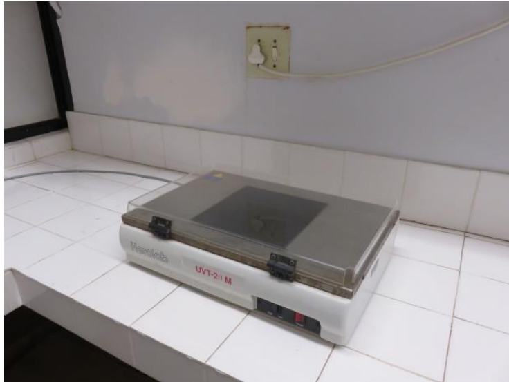
Figure 4.3: An ultraviolet transilluminator (Herolab UVT-20 M) used to visualise PCR products. (Photograph by Raphahlelo ME)
