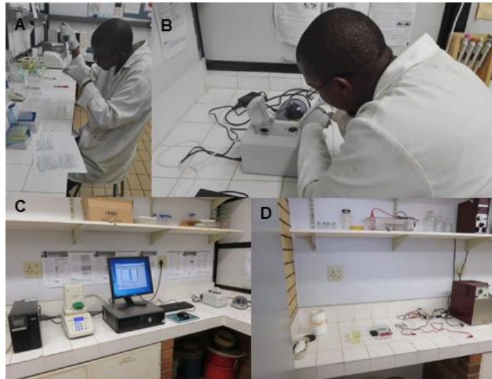
Figure 4.1: A – DNA extraction, B – Measuring DNA concentration using the Thermo Scientific NanoDrop™ version 2000, C – PCR amplification and D – Preparation of gel loading dye. (Photographs by Mangena T)
