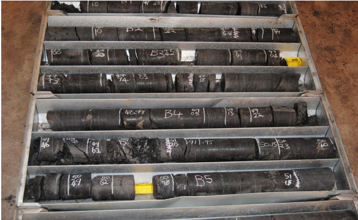
Figure 6.2: Photograph of borehole OV125156 showing coal (C) that varies from dull heavy coal, bright coal and combination of bright and heavy coal of the Madzaringwe Formation.
