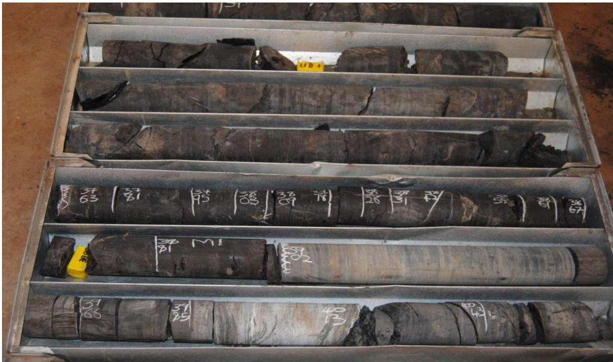
Figure 4.2: Photograph of borehole OV125149 showing shales with thin layer of sandstones and coal of the Madzaringwe Formation.
