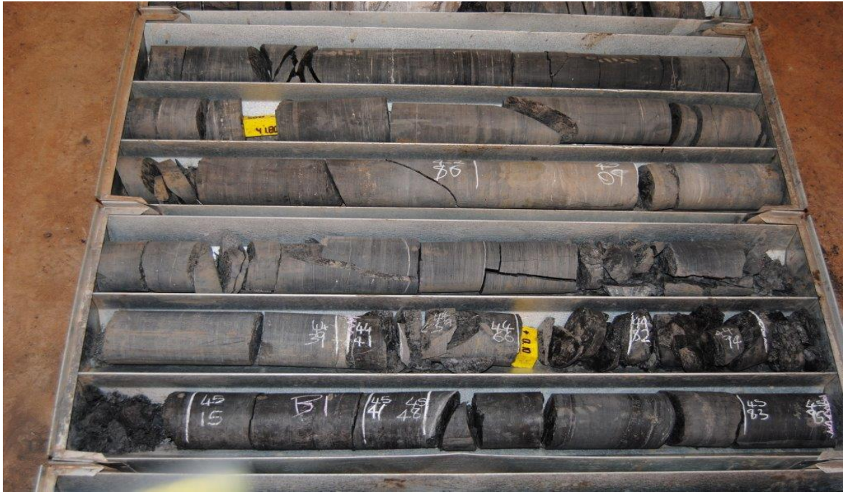
Figure 4.3. Photograph of borehole OV125149 showing lighter to darker colour shales and very bright coal of Madzaringwe Formation.
