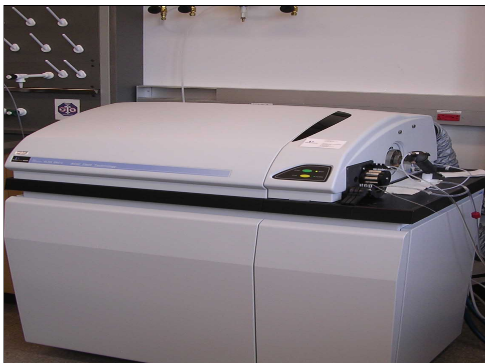
Figure 2.11: Typical ICP-MS from Perkin Elmer
