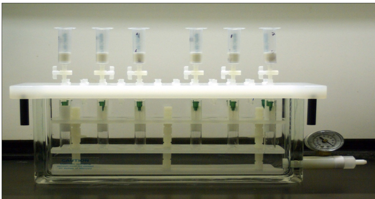
Figure 3.7: The SPE setup
