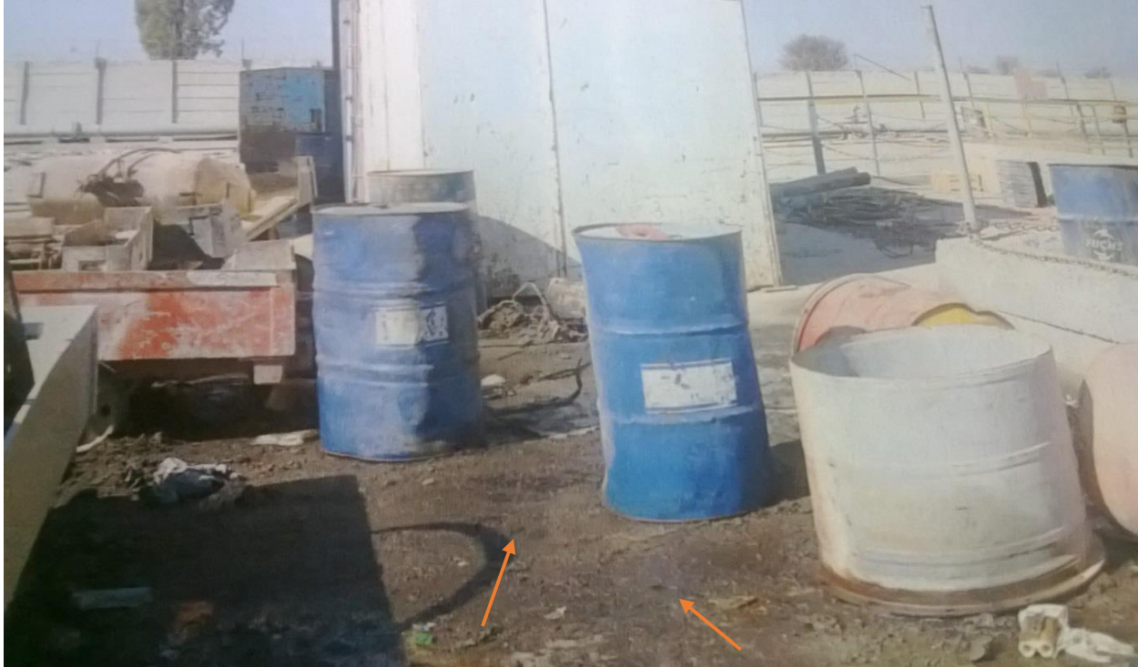
Figure 4.3: Oil spillage in MPM facility (Thovhakale, 2015)
