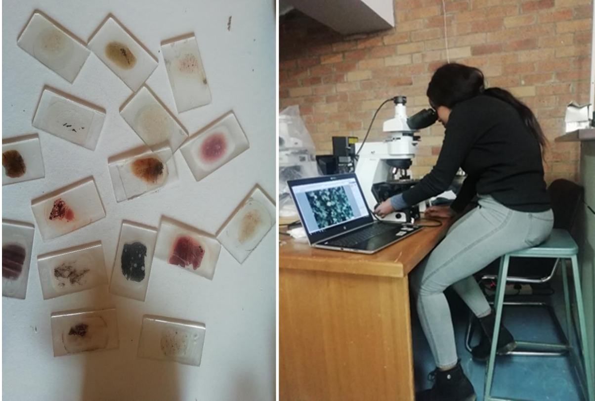
Figure 3.1: Photograph showing analysis of thin section under a Nikon eclipse petrological microscope with a digital camera.
