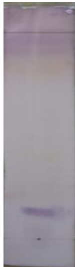
Figure 9.1: Phytochemical profile of the compound isolated from C. bispinosa 's leaves. The chromatogram was run on BEA mobile phase.
