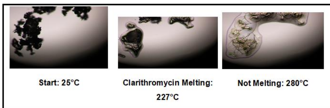
Figure: 4.14: HSM images obtained during heating of clarithromycin and Ac-Di-Sol 1:1 ratio
