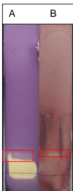
Figure 8.14: The chromatograms E. burkei acetone fractions developed in mobile systems sprayed with 0.2% DPPH in methanol ( A ) for antioxidant activity and sprayed with E. faecalis ( B ) for antibacterial activity.
