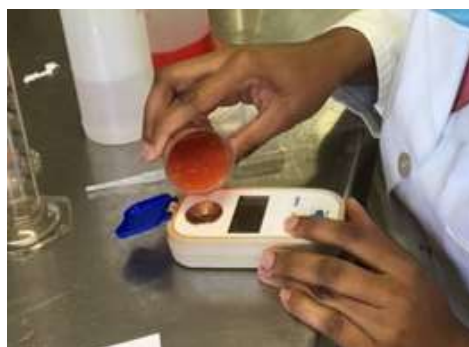
Figure 3.4: Refractometer used to measure tomato juice total soluble solids (TSS)
