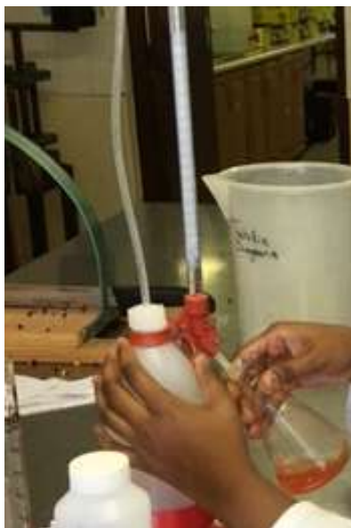
Figure 3.5: Apparatus (burette and flask) used for titration of acid in the tomato juice
