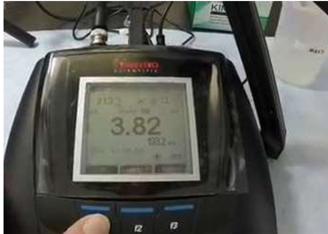
Figure 3.6: Thermo Scientific™ Orion™ Star pH meter used to measure fruit juice pH
