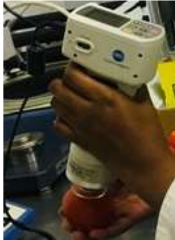
Figure 3.3: Chromameter used to measure colour parameters ( L^* , C^* , a^* , b^* and h^\circ values)
