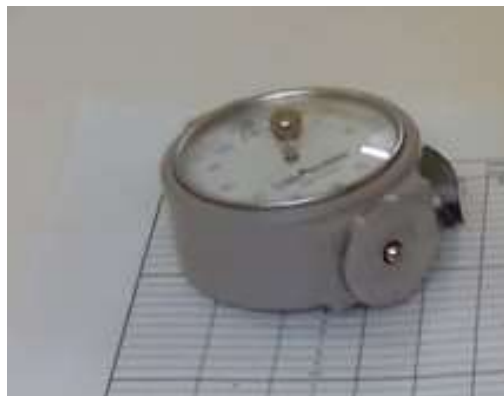
Figure 3.2: Densimeter used to measure tomato fruit firmness
