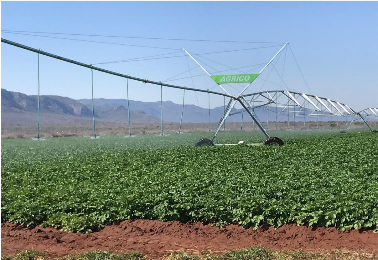
Figure 4. 5: Centre-pivot irrigation system for the potato crop
