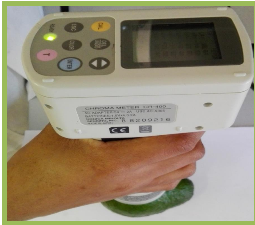
Figure 3.3 Objective colour evaluation of avocado fruit (L, a, b) using a chromameter
