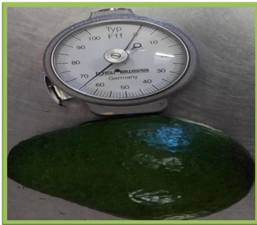
Figure 3.5 Measuring avocado fruit firmness, using a handheld densimeter
