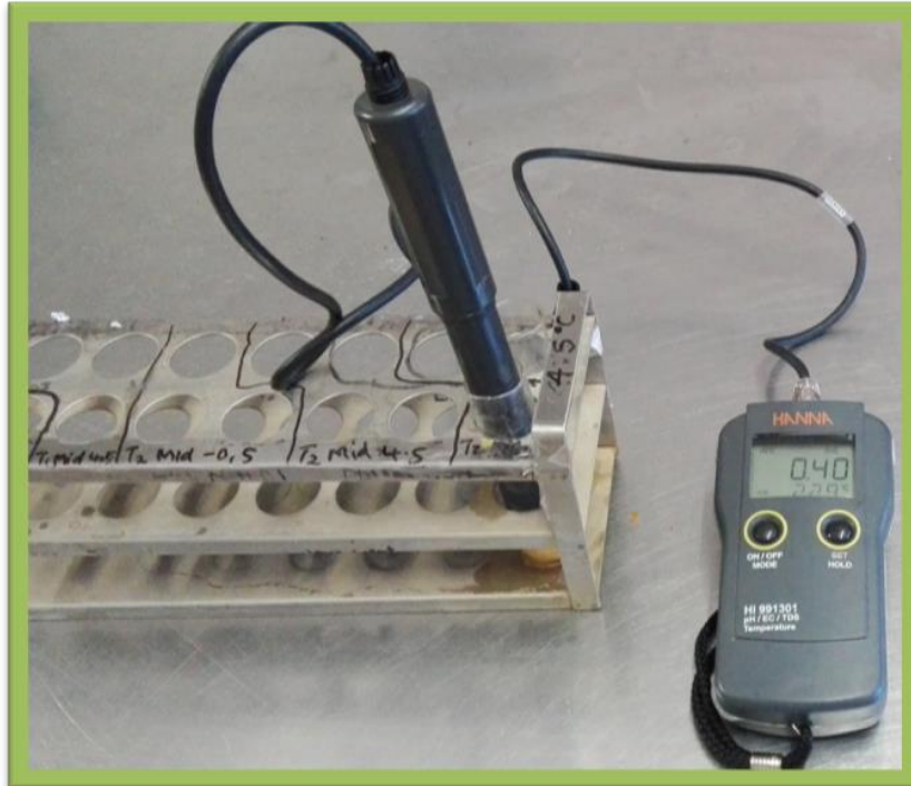
Figure 3.8 Electrical conductivity evaluation of avocado fruit using an EC meter
