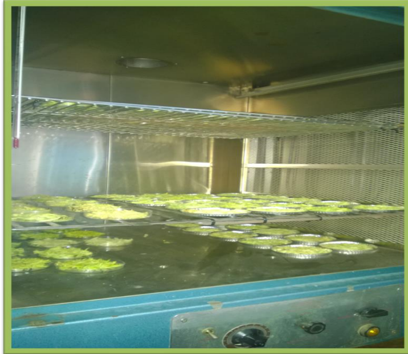
Figure 3.1 Determination of moisture content using the Swarts microwave oven method
