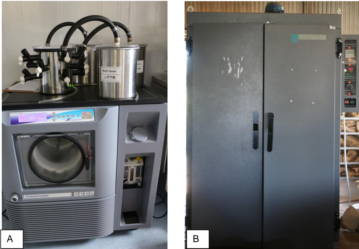
Figure 3.4 Freeze dryer (A) and oven (B) used as some of the drying instruments for Artemisia annua samples in the study.
