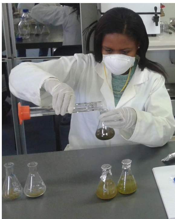
Figure 3.5 Artemisinin extraction from Artemisia annua leaf samples.
