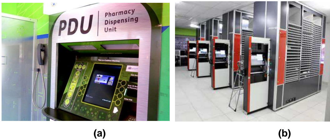
Figure 2.2: The Pharmacy Dispensing Unit: (a) from a patient's view, (b) robotic dispensing system
