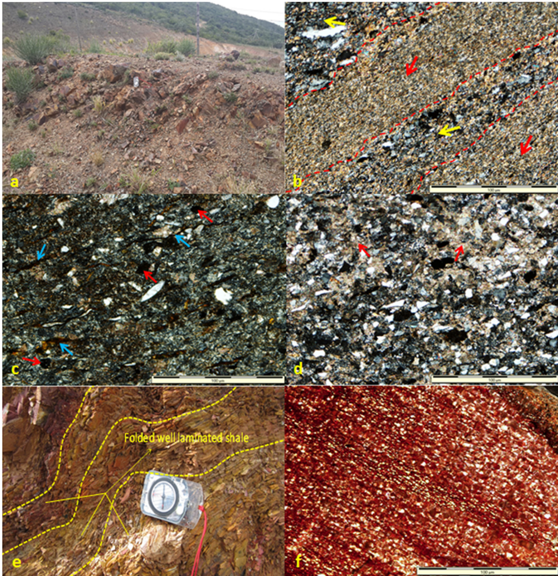
Figure 4: (a) Outcrop photograph showing laminated to thin mudstone and lenticular siltstone (Fss) in the upper part of Prince Albert Formation (Longitude E 26°37'38.1"; Latitude S 33°12'49.5"); (b) thin section photomicrograph of mudrock showing claystone (red arrows) and siltstone (yellow arrows, more than half are clays) layers; (c) thin section photomicrograph of mudrock from the Prince Albert Formation showing siltstone with pyrite (dark area, red arrows) and hematite staining (blue arrow); (d) thin section photomicrograph of mudrock showing calcite replacement of clay matrix and framework grains (brownish area, red arrows); (e) outcrop photograph showing folded well-laminated red stained shale in the upper part of Prince Albert Formation along the Eccca Pass (Longitude E 26°37'38.4"; Latitude S 33°12'59.5"); (f) thin section photomicrograph of mudrock from the Prince Albert Formation showing mud-siltstone with (iron-oxide) hematite staining. Note: The khaki colour shale that is mostly encountered at the upper part of the formation was the product of intense weathering that occurred as a result of tectonic uplift and exposure of the rock to the Earth's surface, leading to the alteration of the original greyish-black colour to khaki colour.
