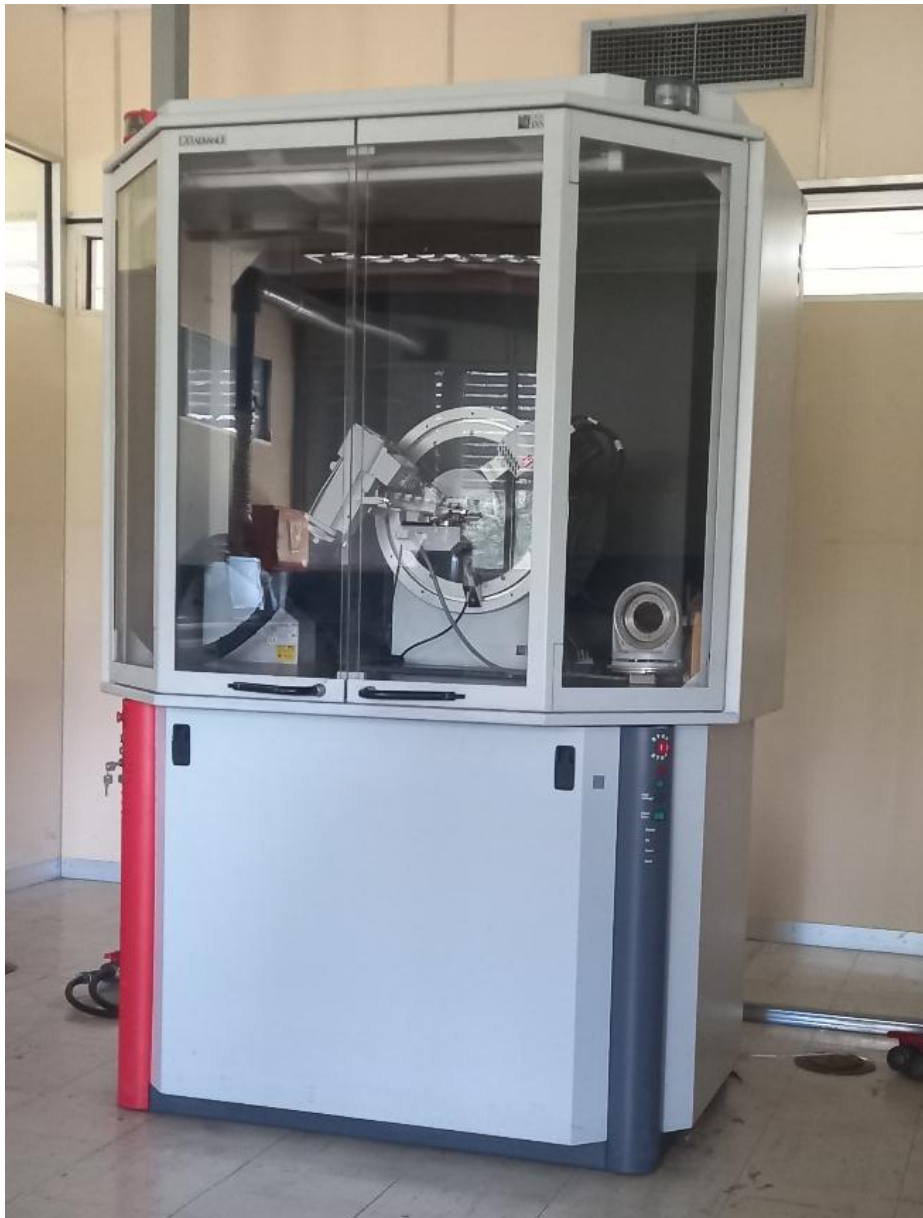
Figure 3. 3: The visualisation of the X-ray diffractometer instrument used to analyse the structural properties of the nanosheets.
