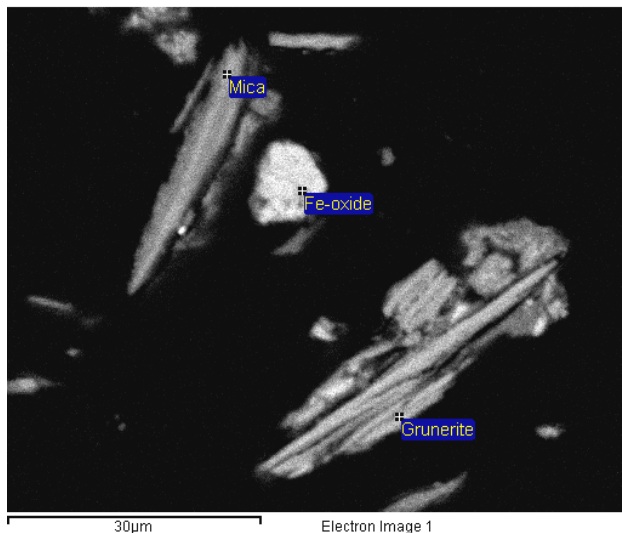
Figure 5.62. BSE images of representative asbestos minerals from sample WP58 cork1
