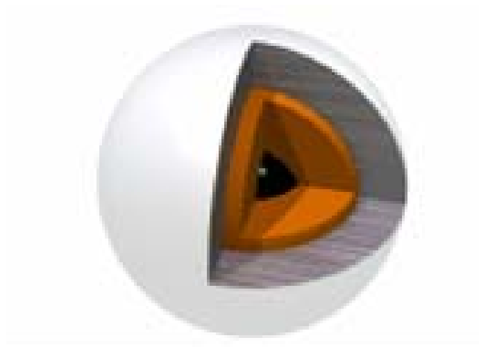
Figure 2.2: The two region approach to calculate defect energies, where the inner black sphere represents a defects, the orange sphere represents the boundary of region I, the grey sphere region IIa , while region IIb tends to infinity [26].
