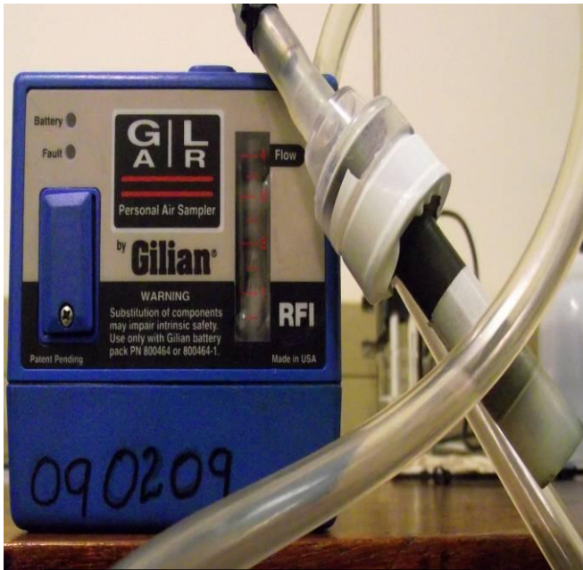
Image 1: Gilian Sampling Pump with filter and cyclone
