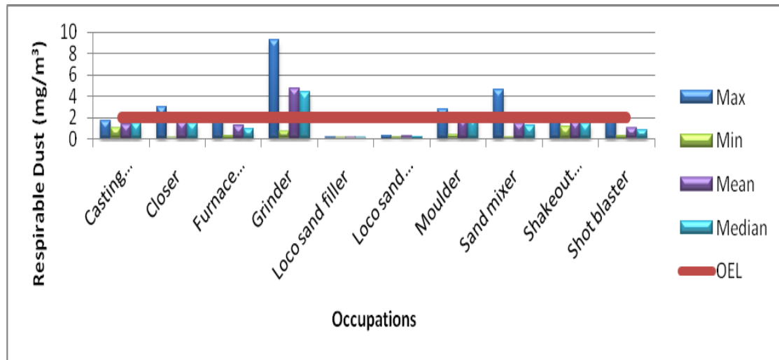
Figure 4.9: Respirable dust exposure per occupation for workers at both foundries (site one and two foundries)
